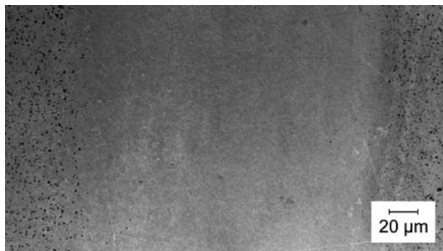
Fig. 3 SEM micrograph (secondary electron image) of the cross-section of a Pd-2 at.% Fe sample after internal oxidation in air for 26 h 42 min at 1273 K
